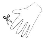
Cut the finger off of a disposable glove to make the top gasket.
