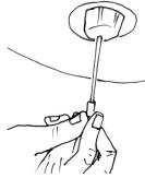
attach 1/4" vinyl rod cap onto the end of toilet float rod.
