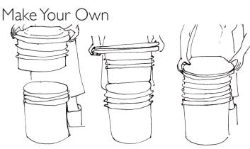
A cut off bucket becomes a flange to fit a seat tightly into a bucket.
