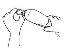
Hold PVC end cap in a clamp or wear gloves to protect your hands. Drill eight 1/16" holes for the water. Angle the drill out away from the middle of the cap.
