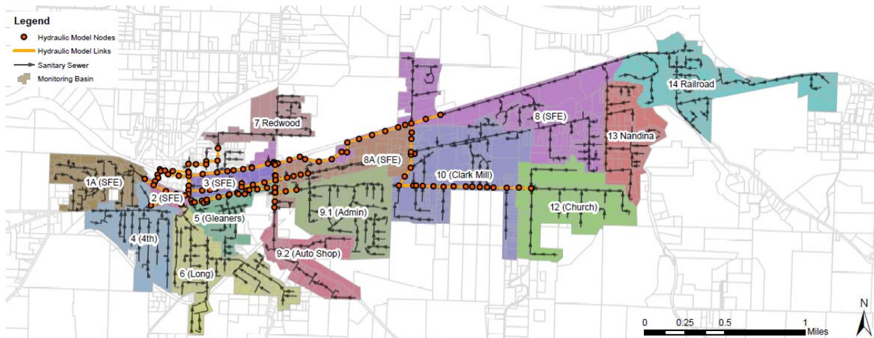
Figure 5-1. Hydraulic modeling network
