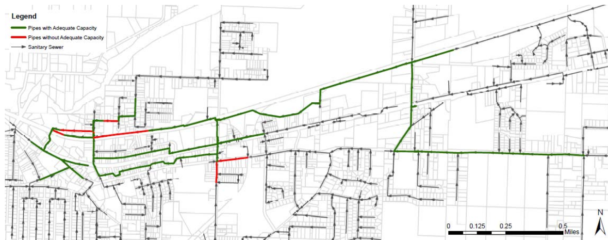
Figure 5-5. Hydraulic modeling results and undersized pipes under future conditions
