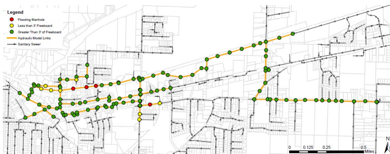
Figure ES-5. Hydraulic modeling results, projected surcharge and overflow locations under future conditions
