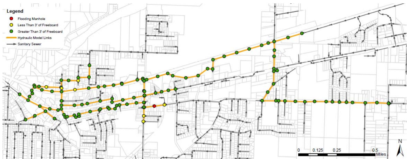
Figure ES-4. Hydraulic modeling results, projected surcharge and overflow locations under existing conditions
