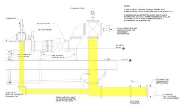
**R:** Yes. The intent is to have ductile iron flanged pipe through the tee that connects the two force mains with valve.
